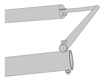
Illustration 3 – Model C wing tip tube correctly bolted to top of trailing edge, creating a built-in washout of 0.9 degrees. \*
