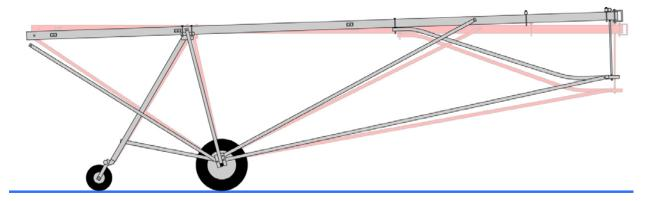
Illustration 4 – Comparison between level boom (shaded red) and negative 2 degree down angle boom.
